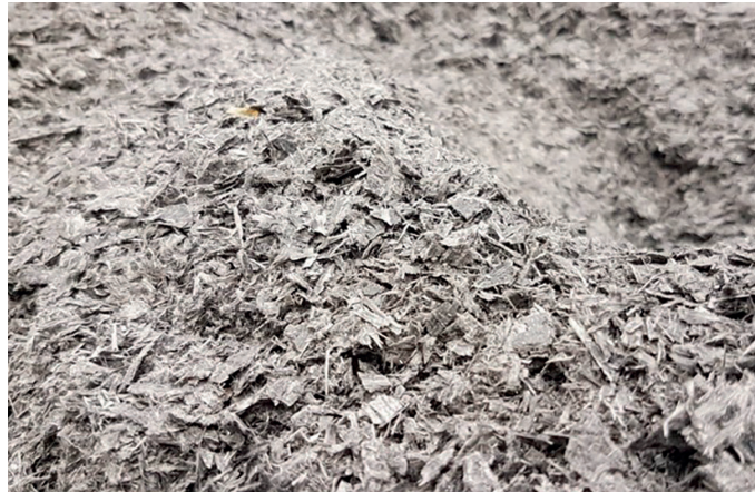
Fig. 1. Shredded Tepex: during shredding, the type of machine used is decisive. Single-shaft shredders in particular are able to produce a homogeneous regrind © Lanxess
